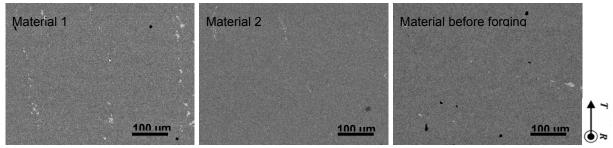
Figure 4: Microstructures of the different materials, comparison of the distribution of carbides and nitrides, in the radial direction.
