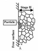
Figure 8 : Schematic representation of the fracture mechanisms for crack initiation from a surface particle [11]
