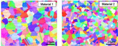
Figure 1 : Grain microstructures observed by EBSD scans with a step of 0.5  $\mu$ m for a) material 1 and b) material 2
