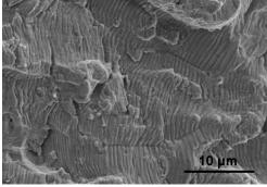
Figure 13 : SEM fractography of the stage II fatigue a) vacuum crack propagation in the fish eye b) air crack propagation beyond the fish-eye.
