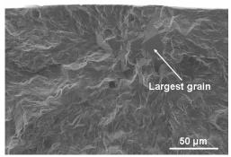
Figure 9 : Fatigue crack initiation sites on microstructure 1 with the biggest mean grains size (11 μm) : Stage I crack initiation across an area of several grains of (a) 70μm of diameter and (b) 150μm of diameter
