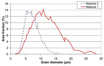
Figure 2: Grain size distributions of the 2 materials calculated from the EBSD data on 1mm<sup>2</sup> zones
