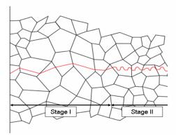
Figure 10 : Schematic representation of the fatigue crack initiation and propagation mechanisms for stage I initiation (for the material with larger grains in the present study)
