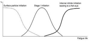
Figure 14: Schematic representation of the relationship between probability to encounter each crack initiation scenario function with the total fatigue life of the specimen for a specific loading value (the relative position of the stage I initiation curve and the internal nitride initiation curve is dependent of a scale effect.
