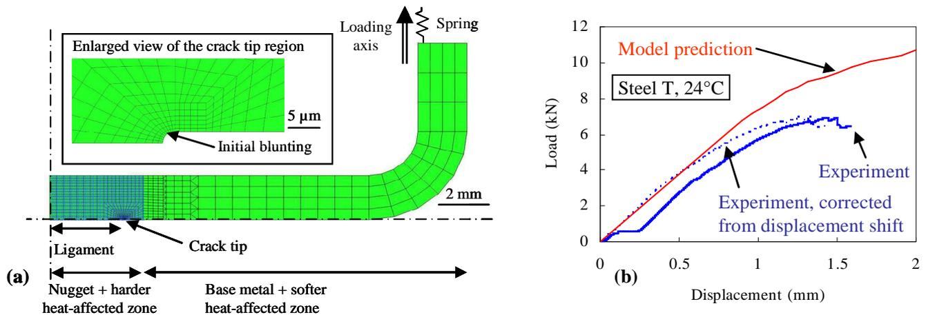
Figure 7. (a) Simplified finite element model and (b) experimental and simulated UXT load vs. displacement curves of Steel T
