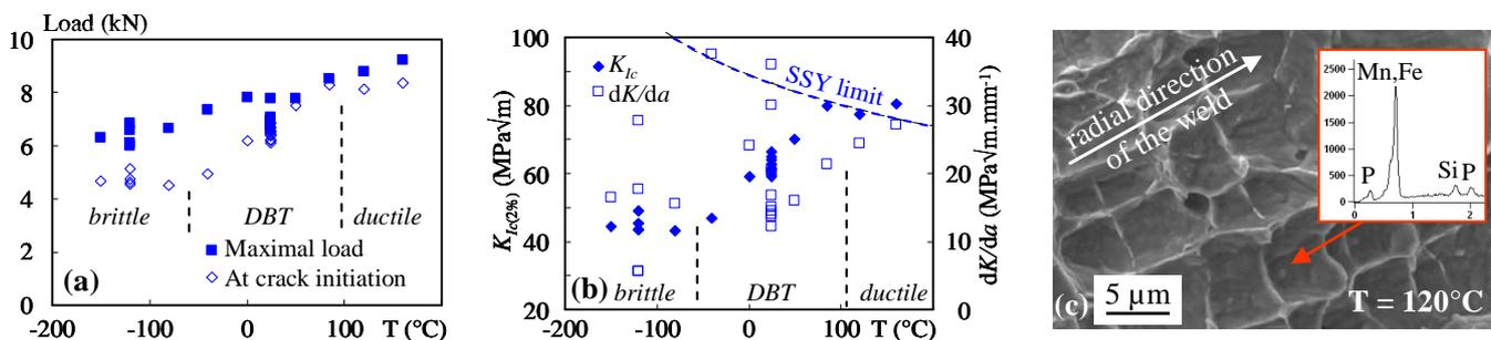
Figure 2. DBT curves for Steel T nuggets: (a) load at crack initiation and weld strength (i.e. maximal load); (b) fracture toughness at crack initiation and crack-extension resistance  $dK/da$ . c) Detailed view of ductile fracture and EDS analysis of precipitates located within dimples (red arrow)
