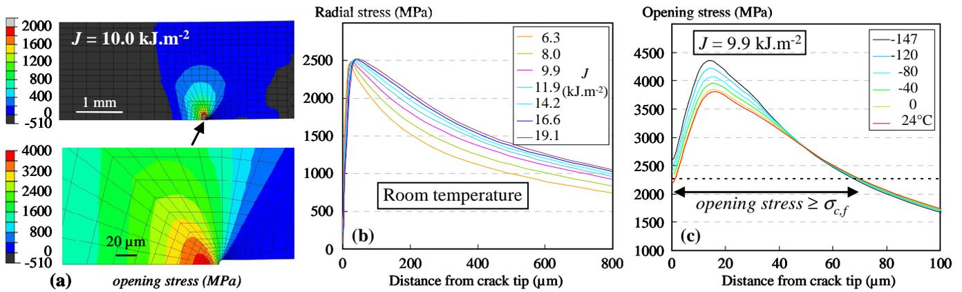
Figure 8. Model predictions of (a) opening stress field at room temperature in the weld, (b) radial stress along the interface as a function of  $J$  and (c) opening stress profile as a function of temperature for Steel D
