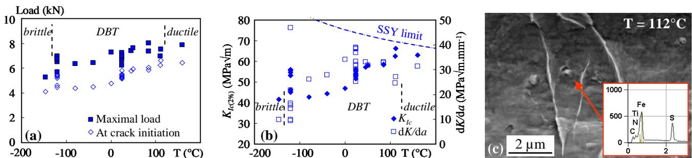
Figure 3. DBT curves for Steel D nugget: (a) load at crack initiation and weld strength; (b) fracture toughness at crack initiation and crack-extension resistance. (c) Ductile dimples nucleated at sulphides
