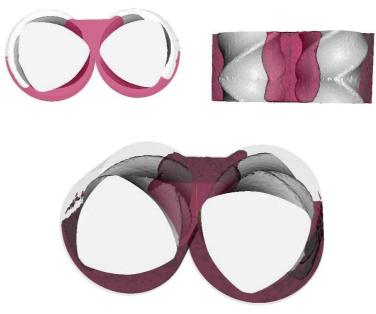
Figure 2: Free surface position in a batch mixer.
