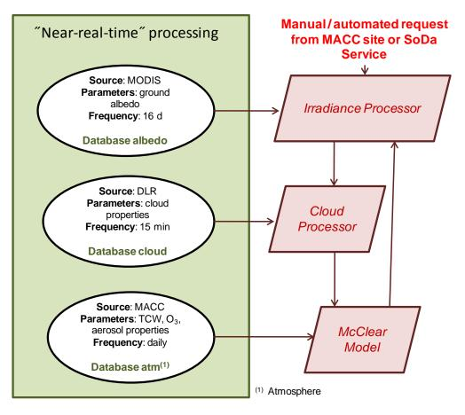
Figure 10.1. Schematic representation of the workflow of the MACC-RAD Service for computing irradiance products. The three databases are part of the HelioClim-4 database.
