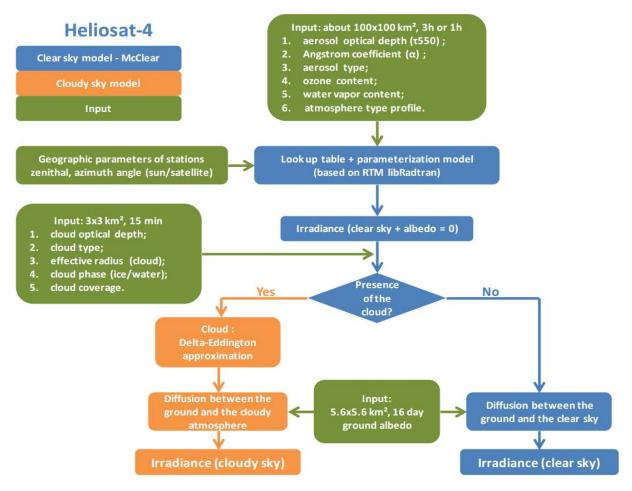
Figure 9.1. Schematic view of the Heliosat-4 method
