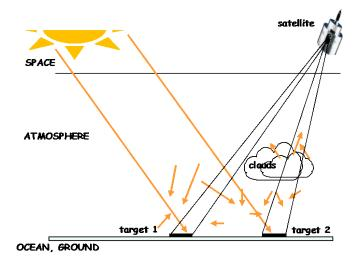
Figure 6.1. Measurement principle as used in cloud-index methods
