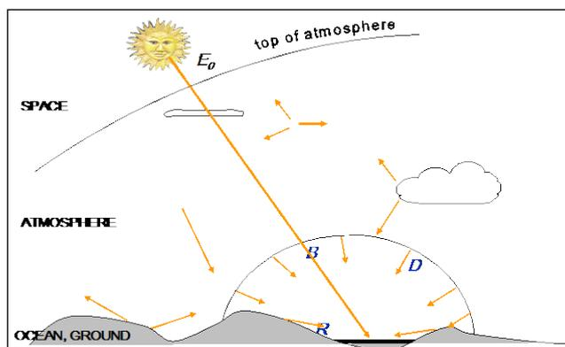
Figure 7.3. Incident irradiance in a complex terrain. B: direct irradiance; D: diffuse irradiance; R: irradiance reflected by nearby terrain
