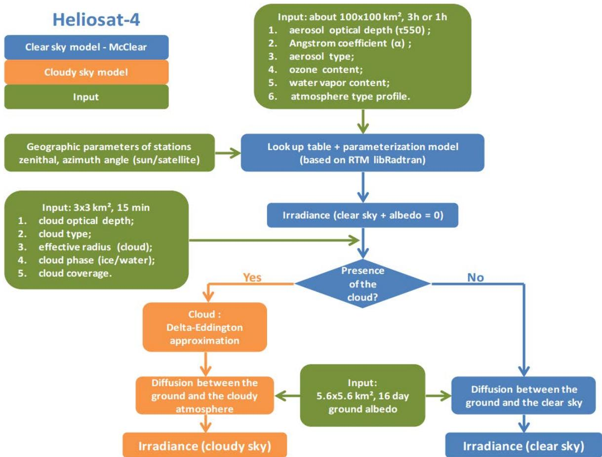
Figure 9.1. Schematic view of the Heliosat-4 method
