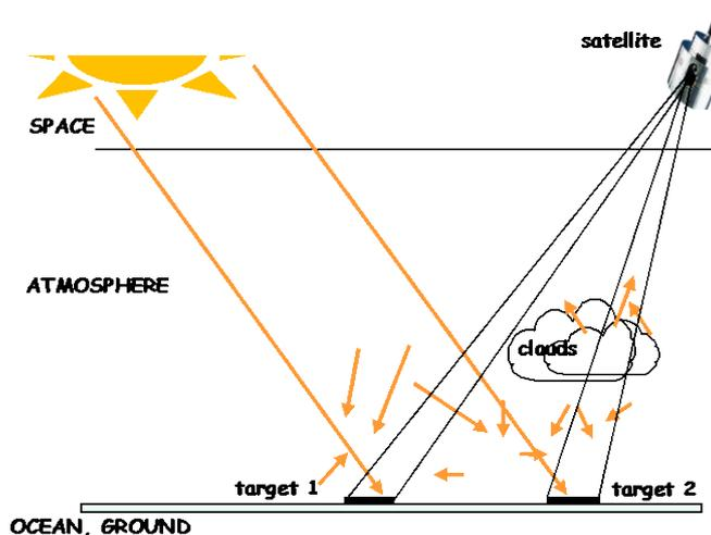
Figure 6.1. Measurement principle as used in cloud-index methods
