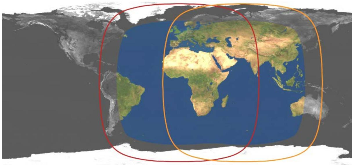
*Figure 5.1: Field of view of the Meteosat Prime (in red) and Meteosat East (in orange). The blue area denotes the part of the area where irradiances can be computed; this is the coverage of the database SOLEMI.*
