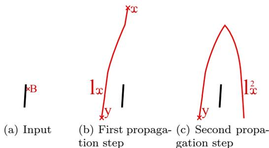
**Fig. 4** A black and white cherry: illustration of the barycentric diameter. Point B is barycentre of the  $CC$  and the starting point of the first propagation ( $x$ ) is the farthest point from B. Then, the first propagation gives  $l_x$  and the second propagation, starting from  $y$ , leads to a much better approximation of the geodesic diameter:  $l_x^2$ .
