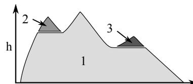
**Fig. 11** Illustration of the algorithm principle for a one-dimensional signal with three local maxima. The components in light grey (marked by one) are analysed first, followed by the components marked by 2 and 3.
