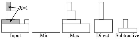
**Fig. 1** Results of an attribute thinning with different filtering rules. From left to right: input signal with two CCs that fulfil the criterion  $\chi$  (in grey), min, max, direct and subtractive rules.
