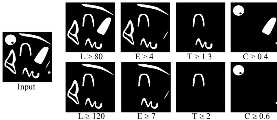
**Fig. 7** Filtering with geodesic attributes criteria: (first column) initial image, (second column) barycentric diameter thinnings, (third column) geodesic elongation thinnings, (fourth column) geodesic tortuosity thinnings and (fifth column) geodesic circularity thinnings.
