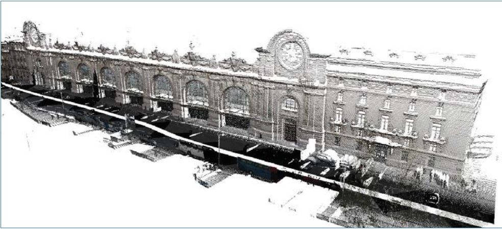
Fig. 2. MLS point cloud – northern façade of Musée d'Orsay
