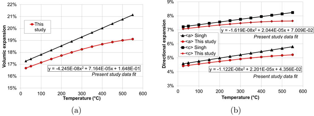
Figure 5: Calculated (a) volumetric expansion and (b) directional expansion induced by  $\delta$  hydrides precipitation following PLTS assumption and comparison with Singh et al. [23]. The indicated equations with  $y$  the directional expansion and  $x$  the temperature in Celsius degrees were obtained using a least-squares fitting method.
