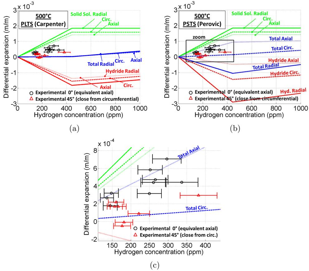
Figure 9: Contribution of hydrogen in solid solution and hydrides to the expansion of samples heated at 500°C with (a) PLTS or (b) PSTS assumption. The Kearns factors are  $f_r = 0.6, f_\theta = 0.3$  and  $f_z = 0.1$ . Figure (c) is a close-up view of Figure (b).
