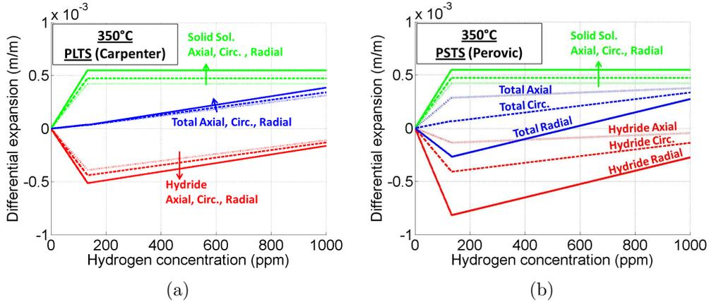
Figure 10: Contribution of hydrogen in solid solution and hydrides to the expansion of samples heated at 350 °C with (a) PLTS or (b) PSTS assumption. The Kearns factors are  $f_r = 0.6, f_\theta = 0.3$  and  $f_z = 0.1$ .
