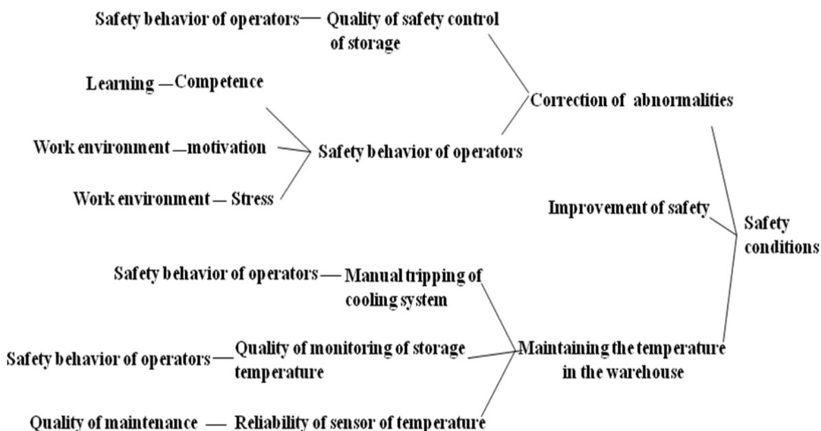
**Figure 11:** Cause tree showing the variable “safety conditions”.
