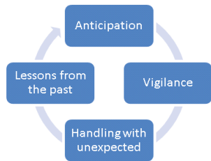
Figure 2. Risk management process according to Wybo. This cycle is the basis for control systems.
