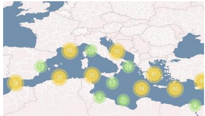
Figure 3. Cluster method to display ships position with an OpenLayers map (FishEye, MINES ParisTech - CRC).
