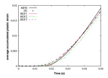
**Fig. 3.** Average acumulated plastic strain in the matrix after tensile deformation up to 5% for a volume fraction of the inclusions equal to 15% and at the strain rate of  $1 \text{ s}^{-1}$ .
