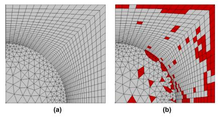
Fig. 1. 2D unit cell representation of a two-phase composite with periodic microstructure under axisymmetric loading: (a) full domain, (b) reduced domain in red. (For interpretation of the references to colour in this figure legend, the reader is referred to the web version of this article.)
