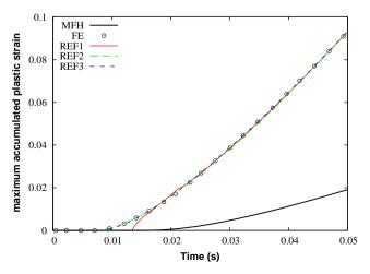
**Fig. 4.** Maximum accumulated plastic strain in the matrix after tensile deformation up to 5% for a volume fraction of the inclusions equal to 15% and at the strain rate of  $16^{-1}$
