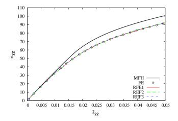
**Fig. 2.** Finite-element, incrementally affine homogenization, and a priori hyper reduction results of the stress–strain curves in tension test at the strain rate of 1 s<sup>-1</sup> for a volume fraction of inclusions equal to 15%.
