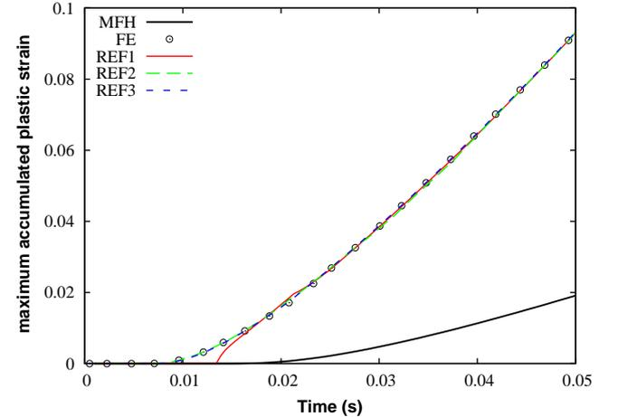
**Fig. 4.** Maximum accumulated plastic strain in the matrix after tensile deformation up to 5% for a volume fraction of the inclusions equal to 15% and at the strain rate of 1 s<sup>-1</sup>.
