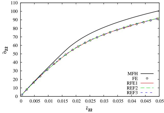
**Fig. 2.** Finite-element, incrementally affine homogenization, and a priori hyper reduction results of the stress–strain curves in tension test at the strain rate of 1 s<sup>-1</sup> for a volume fraction of inclusions equal to 15%.
