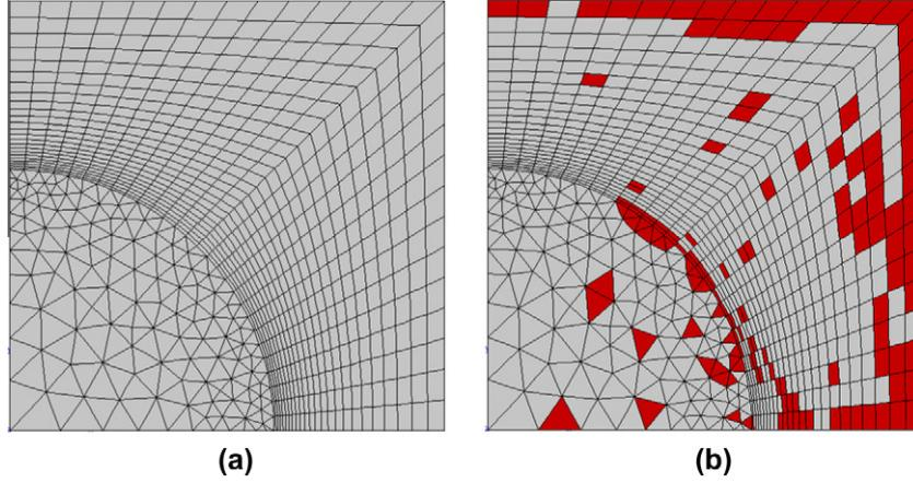
**Fig. 1.** 2D unit cell representation of a two-phase composite with periodic microstructure under axisymmetric loading: (a) full domain, (b) reduced domain in red. (For interpretation of the references to colour in this figure legend, the reader is referred to the web version of this article.)
