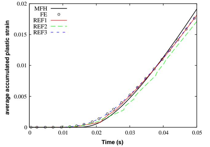
**Fig. 3.** Average accumulated plastic strain in the matrix after tensile deformation up to 5% for a volume fraction of the inclusions equal to 15% and at the strain rate of 1 s<sup>-1</sup>.
