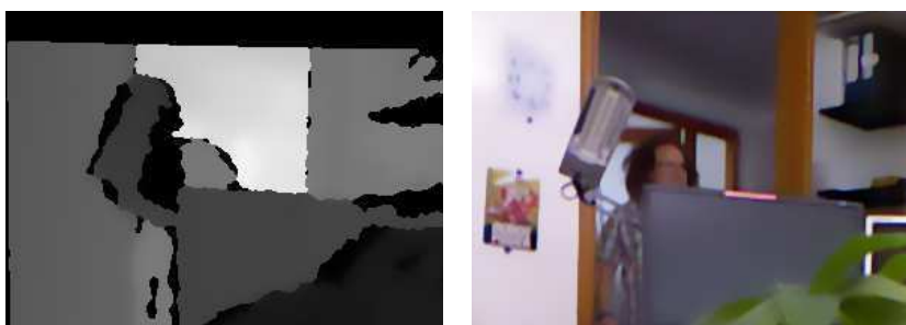
FIGURE 6. Marginal bilateral filtering of RGB and Depth images of Fig. 1. The four components have been filtered with \sigma_s = 5 and \sigma_r = 0.1 .
