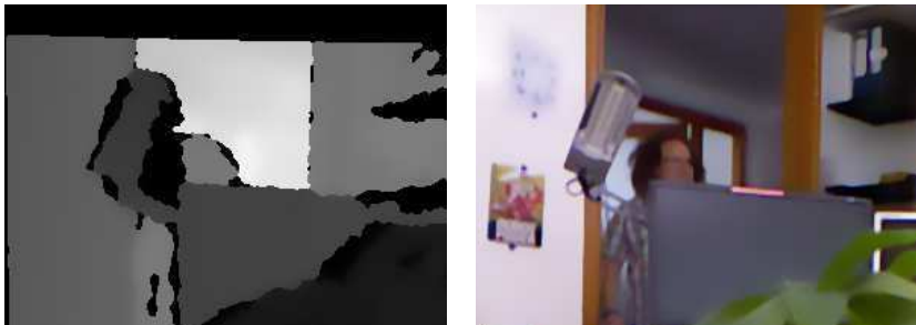
FIGURE 6. Marginal bilateral filtering of RGB and Depth images of Fig. 1. The four components have been filtered with \sigma_s = 5 and \sigma_r = 0.1 .
