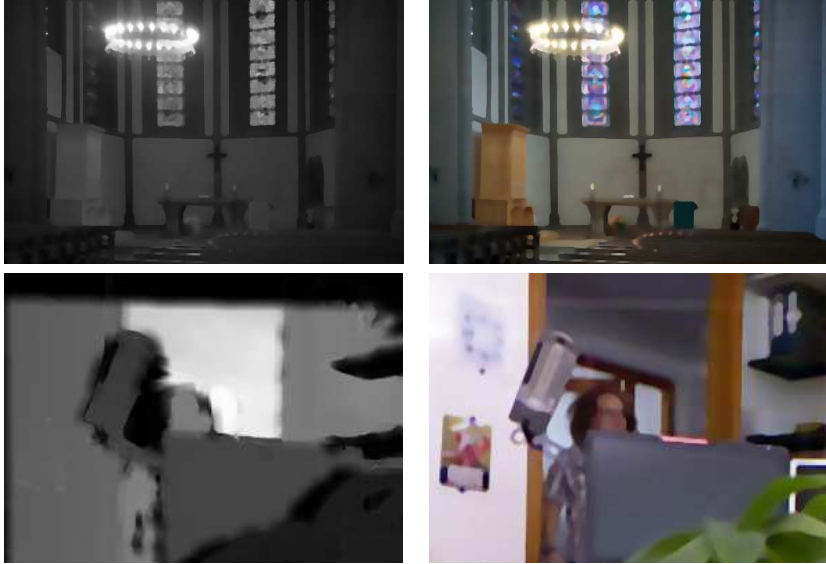
FIGURE 5. Quaternion bilateral filtering BL(f_{\mathbf{q}}) of RGB+NIR and RGB+Depth images of Fig. 1. In both cases it consists in Log-Euclidean mean averaging, with \sigma_s = 5 and \sigma_r = 0.1 .
