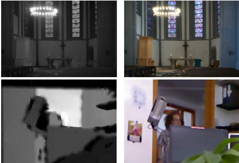
FIGURE 5. Quaternion bilateral filtering BL(f_{\mathbf{q}}) of RGB+NIR and RGB+Depth images of Fig. 1. In both cases it consists in Log-Euclidean mean averaging, with \sigma_s = 5 and \sigma_i = 0.1 .
