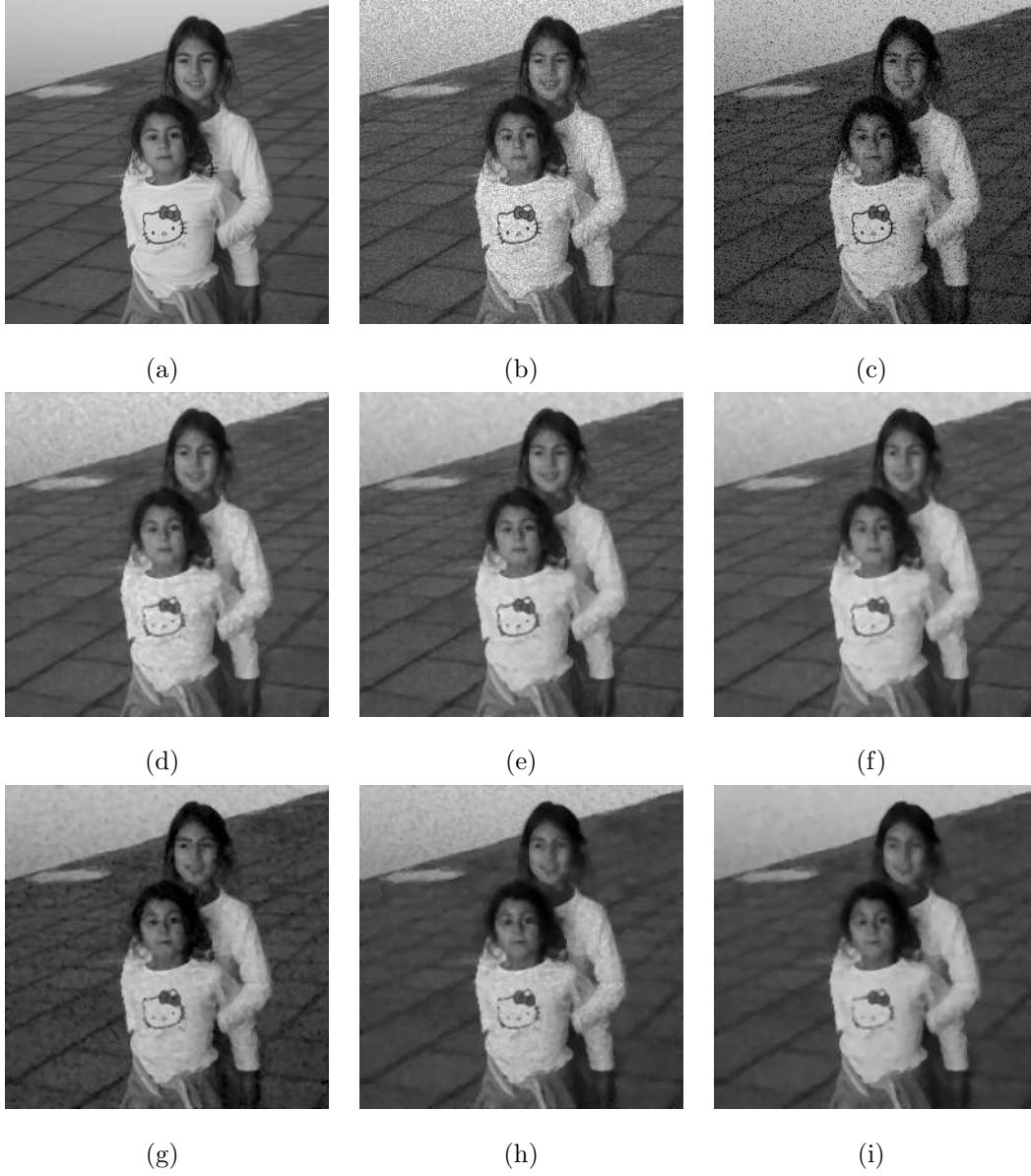
Figure 10: Image denoising using generalised morphological nonlinear diffusion \xi(x, y; t; P) : (a) original unnoisy image, f ; (b) image corrupted with speckle noise \sigma = 0.01 , f' ; (c) image corrupted with asymmetric impulse noise \sigma = 0.1 , f'' ; (d) restoration of image (b) using \xi(x, y; t = 5; P = 0)(f') ; (e) restoration of image (b) using \xi(x, y; t = 5; P = -3)(f') ; (f) restoration of image (b) using \xi(x, y; t = 5; P = 3)(\xi(x, y; t = 5; P = -3)(f')) ; (g) restoration of image (c) using \xi(x, y; t = 5; P = 0)(f'') ; (h) restoration of image (c) using \xi(x, y; t = 5; P = -5)(f'') ; (i) restoration of image (c) using \xi(x, y; t = 5; P = 5)(\xi(x, y; t = 5; P = -5)(f'')) .
