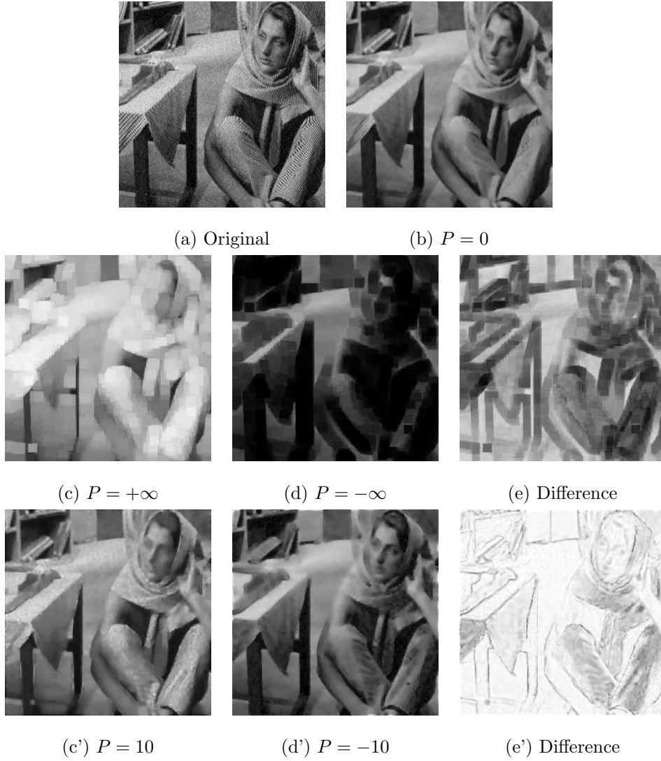
Figure 6: Generalised morphological Perona and Malik diffusion \xi(x, y; t; P) at scale t = 5 (regularization parameter \sigma = 0.5 ): (a) original image, (b) standard nonlinear diffusion, (c)/(d) standard dilation/(d) standard erosion, (e) image difference between dil./ero. (gradient), (c')/(d') pseudo-dilation/erosion by counter-harmonic nonlinear diffusion, (e') image difference between pseudo-dil./ero.
