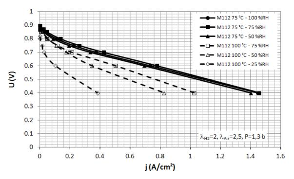
**Figure 9.** Polarization curves obtained for M112, at 75 °C (solid lines) and 100 °C (dashed lines), between 25 and 100% relative humidity.
