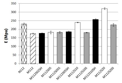
**Figure 7.** Elastic modulus measured for the different membranes by Dynamics Mechanical Analysis at 25 °C and 1 Hz.
