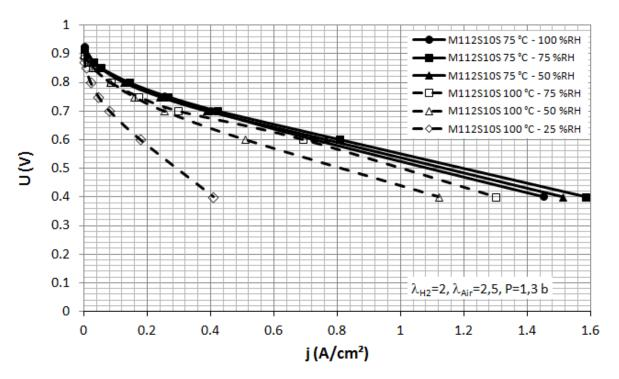
**Figure 11.** Polarization curves obtained for M112S10S, at 75  $^{\circ}$ C (solid lines) and 100  $^{\circ}$ C (dashed lines), between 25 and 100% relative humidity.
