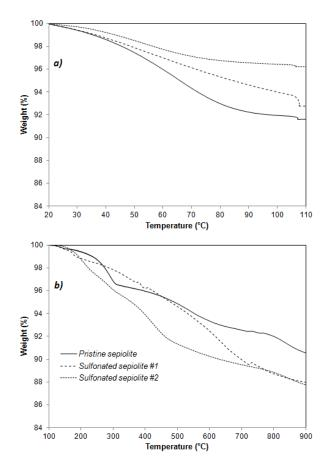
**Figure 3:** TGA under nitrogen of pristine sepiolite and sulfonated sepiolites (protocols #1 and #2), a) from 25 to 110°C at 10°C/min followed by an isotherm at 110°C for 10 min, b) from 110 to 900°C at 10°C/min.
