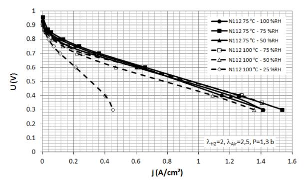
**Figure 8.** Polarization curves obtained for N112, at 75  $^{\circ}$ C (solid lines) and 100  $^{\circ}$ C (dashed lines), between 25 % and 100% relative humidity.
