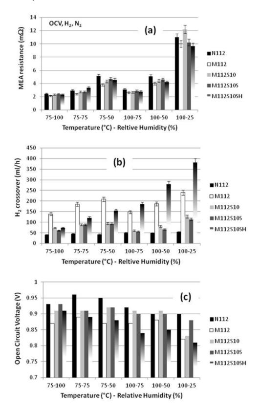
Figure 14. Influence of the temperature and the relative humidity (RH) on the MEA resistance (a), on the  $H_2$  crossover (b) and on the open circuit voltage (c), for the different membranes [from the left to the right: N112 (black), M112 (white), M112S10 (light grey), M112S10S (dark grey) and M112S10SH (gradation)].
