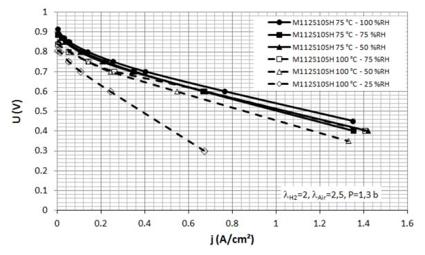
**Figure 12.** Polarization curves obtained for M112S10SH, at 75 °C (solid lines) and 100 °C (dashed lines), between 25 and 100% relative humidity.
