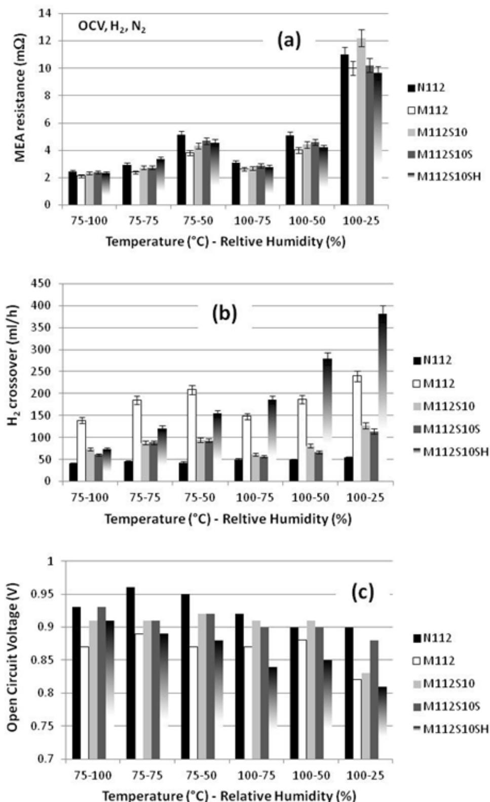
**Figure 14.** Influence of the temperature and the relative humidity (RH) on the MEA resistance (a), on the H<sub>2</sub> crossover (b) and on the open circuit voltage (c), for the different membranes [from the left to the right: N112 (black), M112 (white), M112S10 (light grey), M112S10S (dark grey) and M112S10SH (gradation)].
