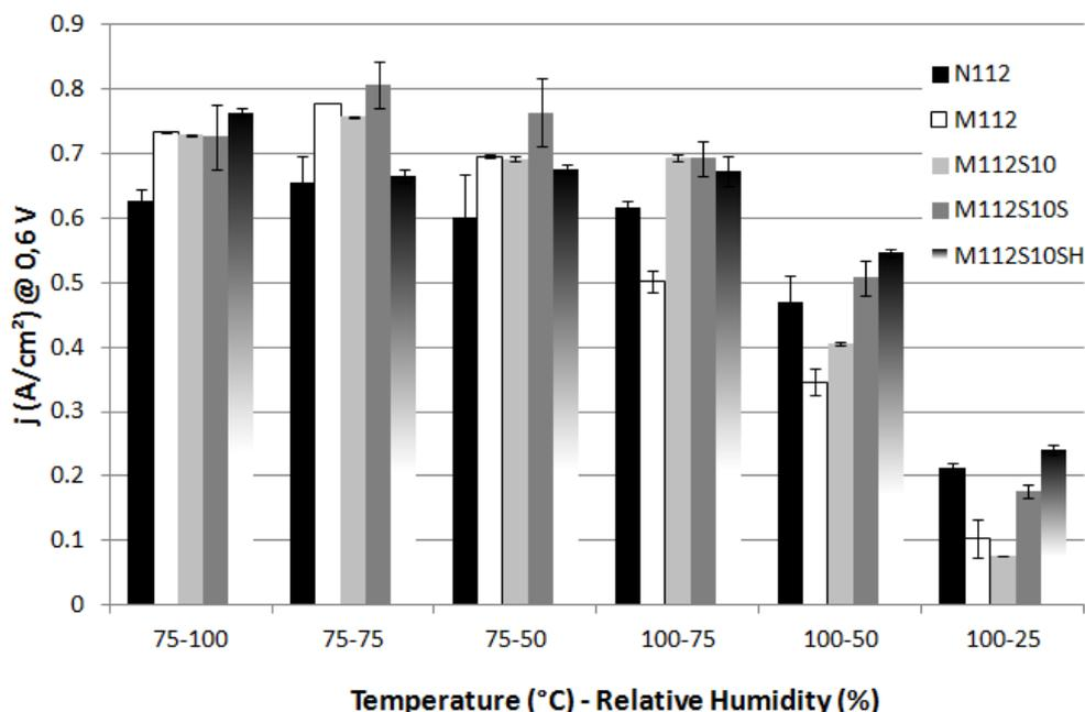
**Figure 13.** Influence of the temperature and the relative humidity (RH) on the current density at 0.6 V for the different membranes: N112 (black), M112 (white), M112S10 (light grey), M112S10S (dark grey) and M112S10SH (gradation), from left to right.
