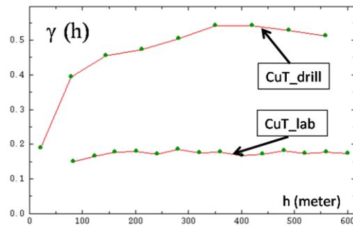
Figure 2 Drill hole and laboratory total grade variograms
