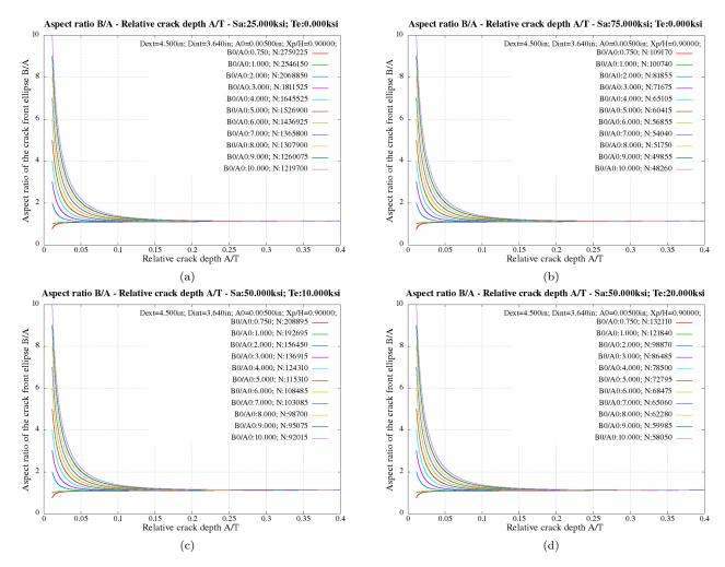
Figure 9: Evolution of the crack ellipse aspect ratio B/A: (a)  $S_a = 25$  ksi and  $T_e = 0$  ksi, (b)  $S_a = 75$  ksi and  $T_e = 0$  ksi, (c)  $S_a = 50$  ksi and  $T_e = 10$  ksi, (d)  $S_a = 50$  ksi and  $T_e = 20$  ksi.
