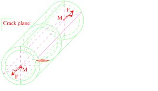
(a) Cracked cylinder and loading
