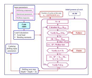
Figure 13: Crack propagation algorithm for rotary drilling operation.
