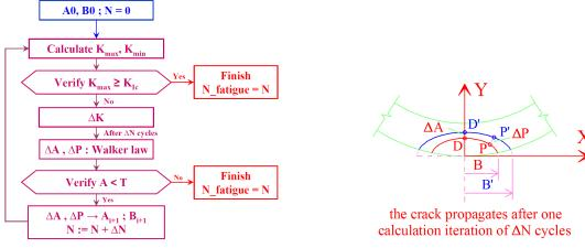
(a) Histogram of crack growth calculating algorithm
