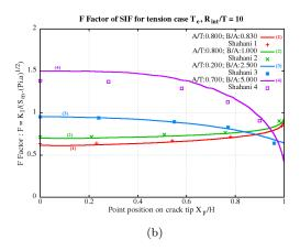
Figure 4: Numerical results - comparisons with the results of Shahani [10]: (a) Bending case, and (b) Tension case
