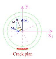
Figure 2: Decomposition of the bending moment
