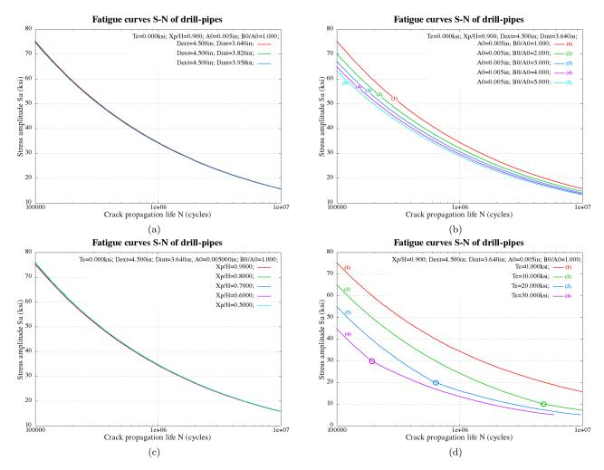
Figure 12: S–N curve computation for drill pipe: (a) different cylinder thicknesses, (b) different initial crack geometries, (c) different choices of the second propagation point P, (d) different tension loadings.
