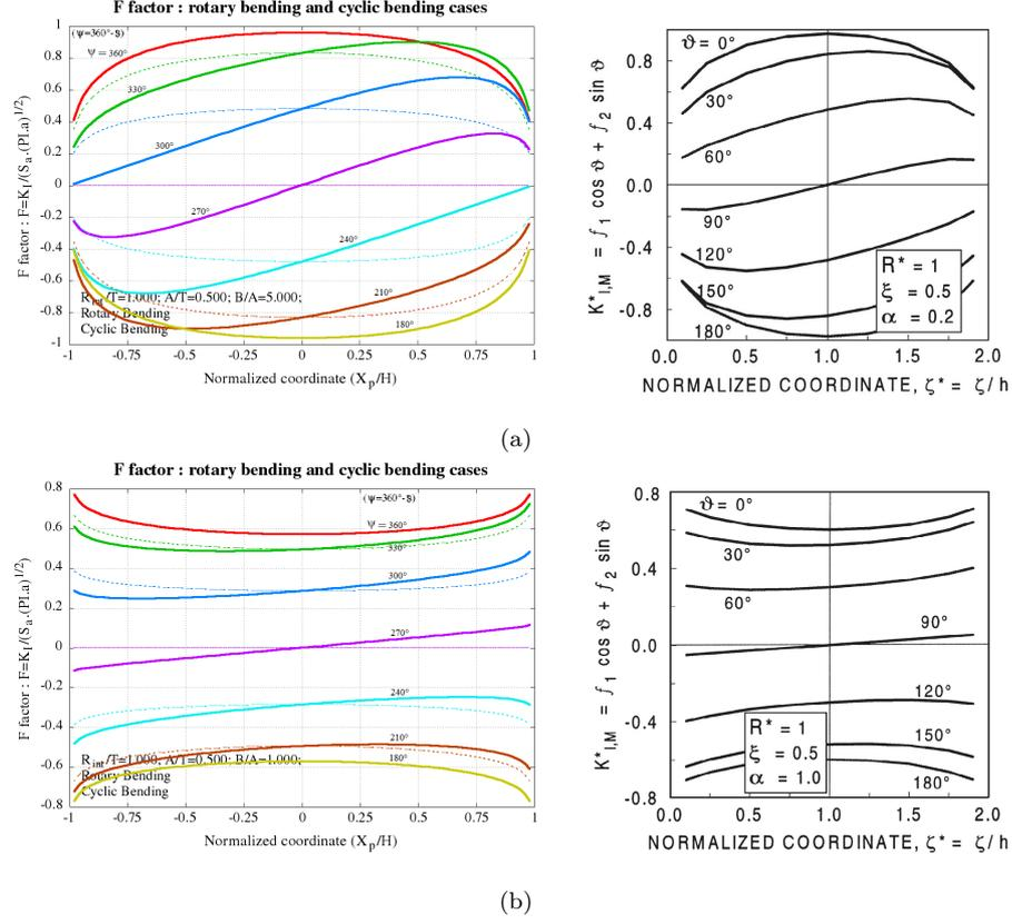
Figure 5: Numerical results - comparisons with the results of Carpinteri [5]: (a)  $R_{int}/T = 1$ ,  $A/T = 0.5$ ,  $B/A = 5$  and different values of  $\psi$ , and (b)  $R_{int}/T = 1$ ,  $A/T = 0.5$ ,  $B/A = 1$  and different values of  $\psi$ .
