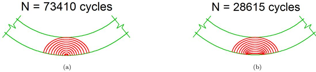
Figure 8: Crack propagation example: (a)  $B_0/A_0 = 1$ , and (b)  $B_0/A_0 = 10$ .
