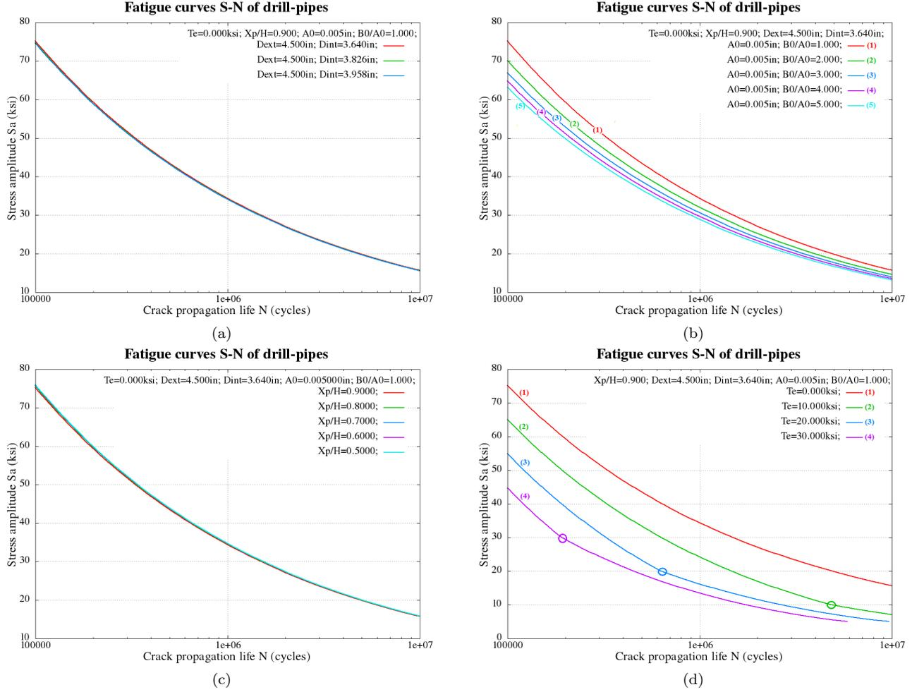
Figure 12: S-N curve computation for drill pipe: (a) different cylinder thicknesses, (b) different initial crack geometries, (c) different choices of the second propagation point  $P$ , (d) different tension loadings.
