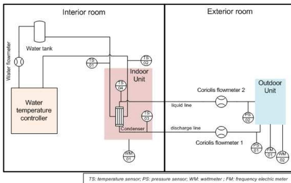
**Figure 1. Flow chart of the test bench**
