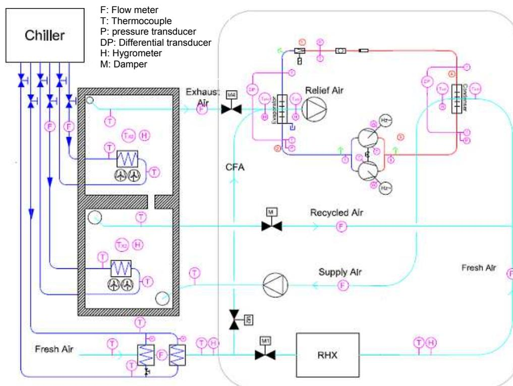
**Figure 4: Schematic lay-out of the test bench**
