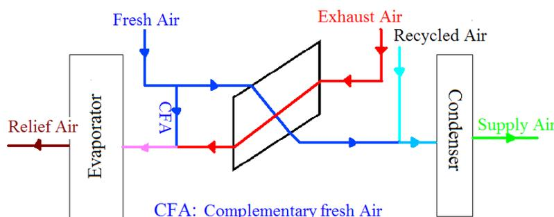
Figure 3: Schematic description of mini-heat pump (MHP)
