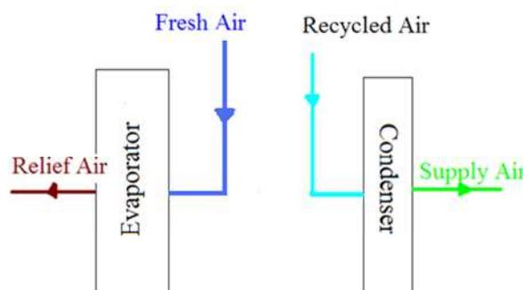
Figure 2: Schematic description of an air-to-air HP
