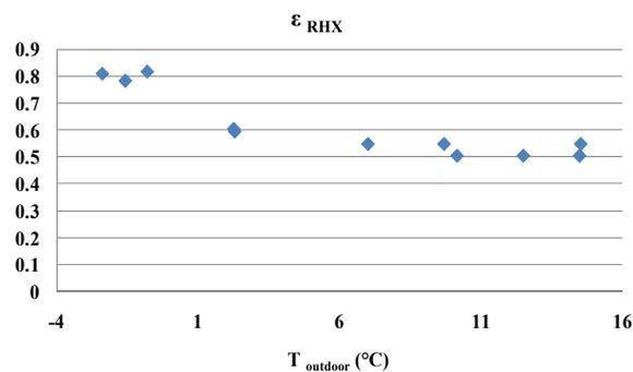
Figure 7: RHX efficiency as a function of the outdoor temperature
