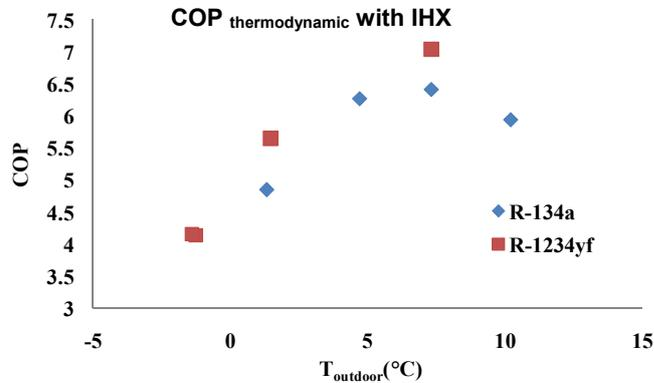
Figure 11: Variation of the COP<sub>thermodynamic</sub> with the outdoor temperature
