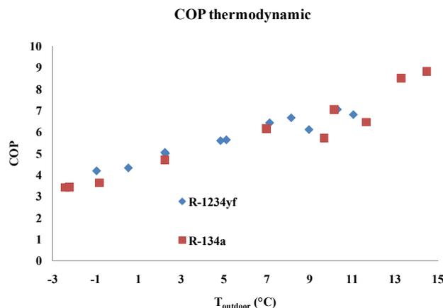
Figure 8: Variation of COP<sub>thermodynamic</sub> according to the outdoor temperature
