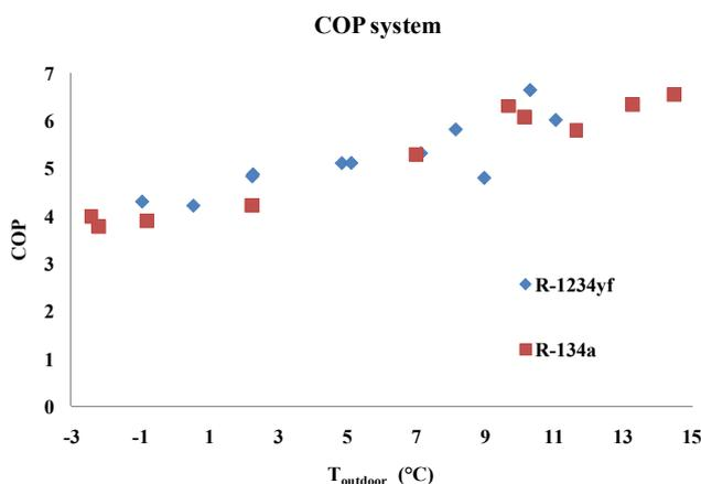
Figure 10: Variation of COP<sub>system</sub> with the outdoor temperature
