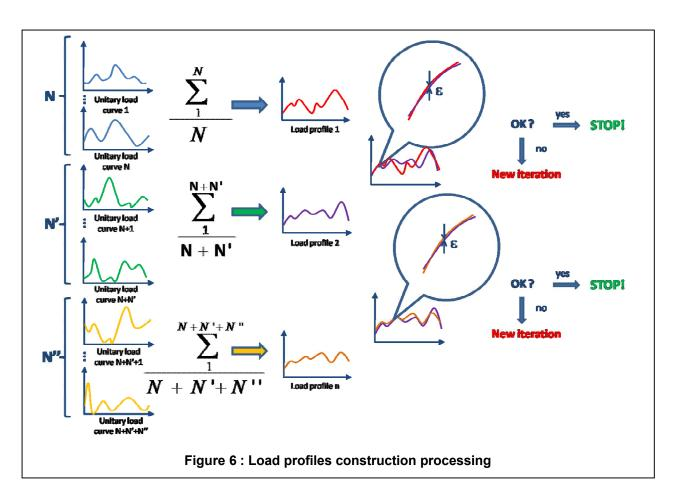
In Figure 6 we schematically expose the way enabling the construction of the load profiles.
