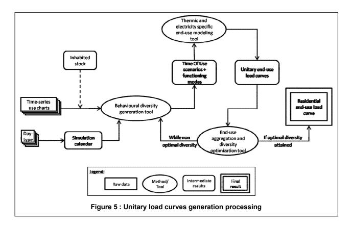
Calculation of the load profiles for each n-tuple and each simulated day
