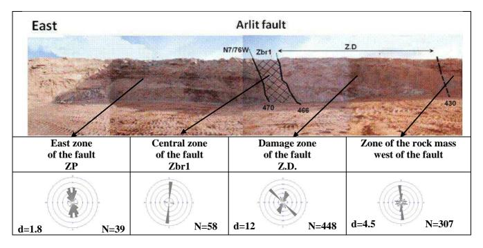
Figure 9: Trench TR1 – South wall: structural zones and for each zone: rose diagram of discontinuity strikes, d=number of discontinuity per metre, N= number of measured discontinuities.
