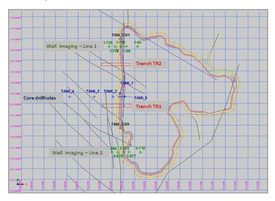
Figure 8: Location of the geotechnical investigation works, Tamgak final pit contour and major faults.
