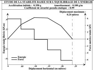
Figure 4: Failure mechanism and calculation of the displacement induced by a dynamic loading due to rock mass blasting (from Fleurisson [7])
