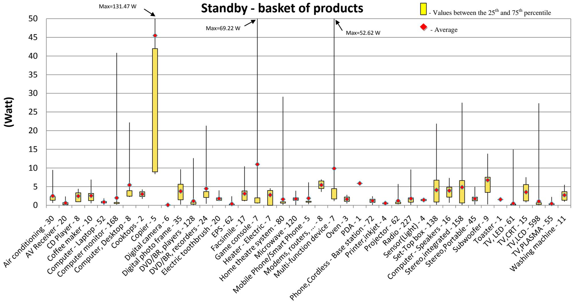
**Figure 7 – Standby input power for basket of products.**
