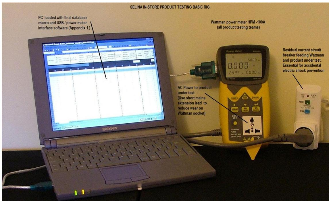
Figure 3 – Illustration of the measurement process.
