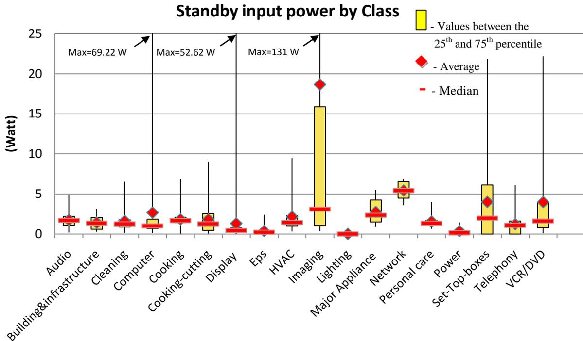
Figure 10 – Standby input power by products class.
