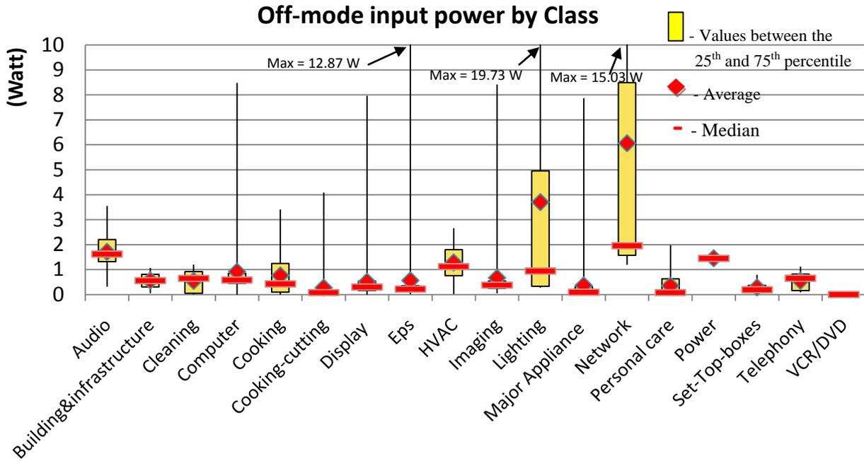
Figure 9 – Off-Mode input power by products class.
