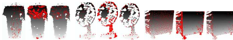
Fig. 3. Detected keypoints on trash can, fan and storage cupboard models with: SID in first column, SC_HK in second column and SC_HK_connex in third column.
