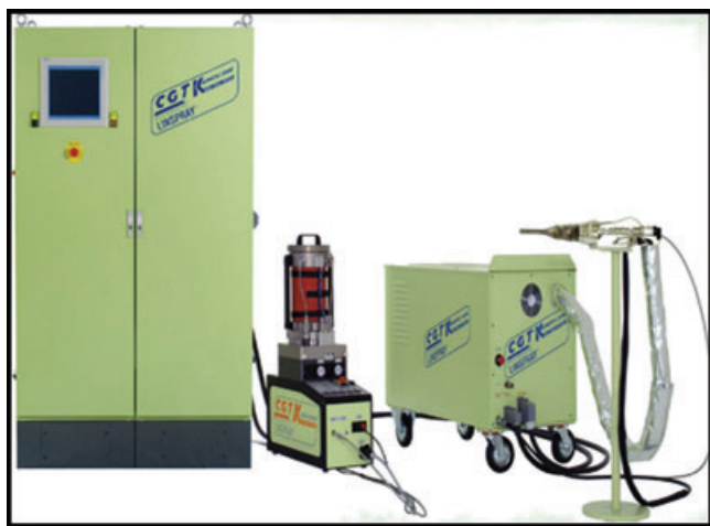
Fig. 2. Cold spray facility at Mines ParisTech (K3000, CGT, Ampfing, Germany).
