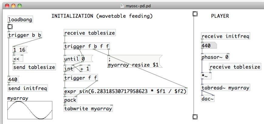
Fig. 2. The `osc.pd` implementation in Pure Data.
