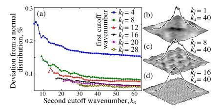
FIG. 5: Mean deviation from the Gaussian distribution (computed over 30 surfaces) with respect to the high cutoff wavenumber  $k_s$ . Various low cutoff wavenumber  $k_l$  are presented by several curves. The Hurst roughness exponent for all surfaces is H = 0.8 and the root mean squared height is rms = 0.1, each surface consists of  $1024^2$  points.
