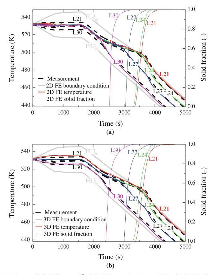
Fig. 4—Comparison of (thick dashed lines) measured<sup>[12]</sup> and (thick plain lines) computed cooling curves with (*a*) 2D and (*b*) 3D solutions of the FE model (without CA coupling). The computed time evolutions of the total fraction of solid phases are added as thin lines.
