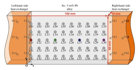
Fig. 1—Schematics of the experimental set-up developed for the solidification benchmark experiment of a Sn-3 wt pct Pb alloy<sup>[11,12]</sup> with position and label of the 62 thermocouples used in the analysis.
