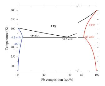
Fig. 2—Phase diagram of the Sn-Pb system as computed with ThermoCalc<sup>[46]</sup> using the PBIN thermodynamic database<sup>[47]</sup> with label of the stability domains of individual phases.
