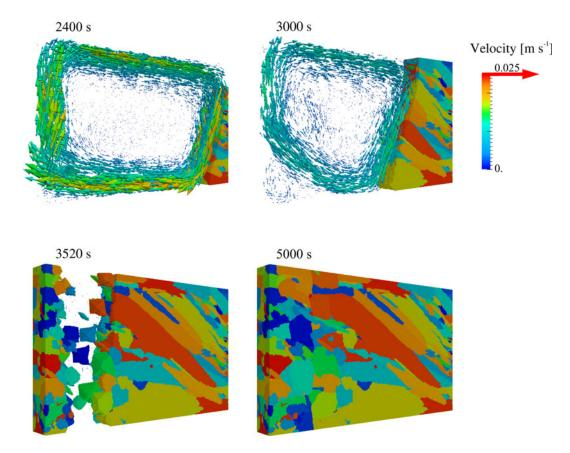
Fig. 5—3D CAFE simulation of the fluid flow and grain structure at different times during solidification of the 100 mm  $\times$  60 mm  $\times$  10 mm Sn-3 wt pct Pb alloy benchmark experiment presented in Fig. 1.
