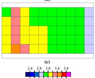
Fig. 9—Final segregation map (a) as observed by X-ray analysis and predicted mid-thickness of the ingot by (b) the 3D FE simulation, and (c) the 3D CAFE simulation. The scale, with units in wt pct, only applies to predicted maps.
