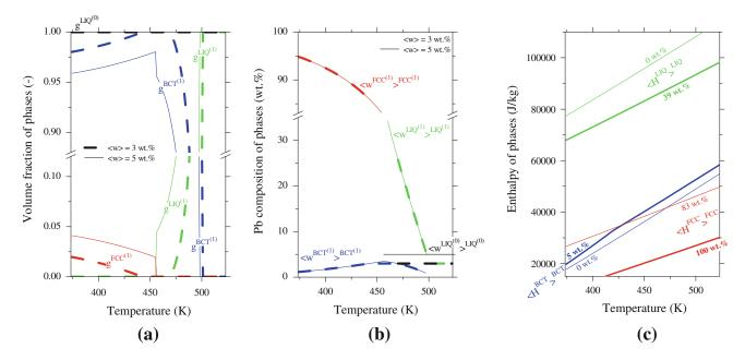
Fig. 3—Tabulations with temperature, for alloys Sn-3 wt pct Pb and Sn-5 wt pct Pb, of phase data: (a) volume fraction, (b) composition, and (c) enthalpy. Data extracted from the PBIN database<sup>[47]</sup> using ThermoCalc<sup>[46]</sup> and assuming full equilibrium.
