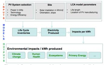
Figure 4: Data inputs, model and outputs results linkage
