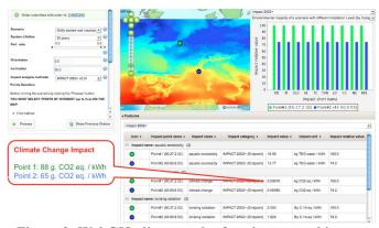
Figure 9: WebGIS client result of environmental impact assessment of a PV system
