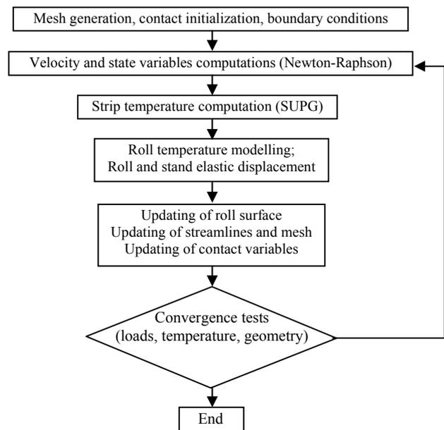
**Figure 3.** General algorithm of the Lam3/Tec3 FEM strip rolling model.
