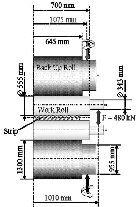
**Figure 5.** The mill structure (4-Hi) and dimensions.
