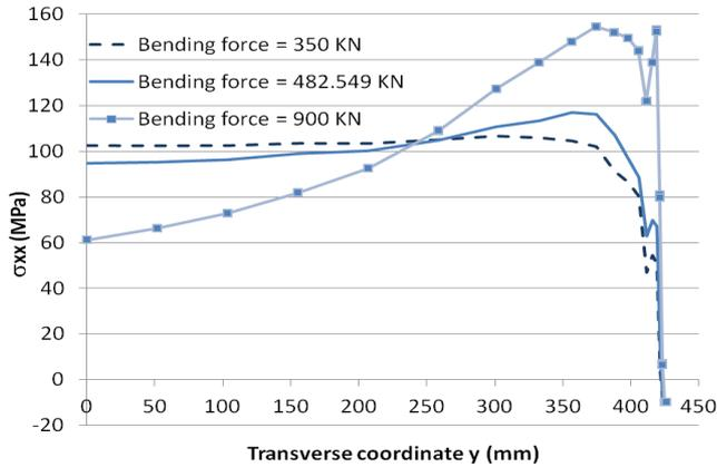
**Figure 13.** The  $\sigma_{xx}(y)$  stress profile for varying bending force and fixed friction coefficient ( $\mu = 0.025$ ).
