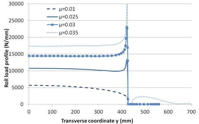
Figure 12. Roll load transverse distribution  $F(y)$ .
