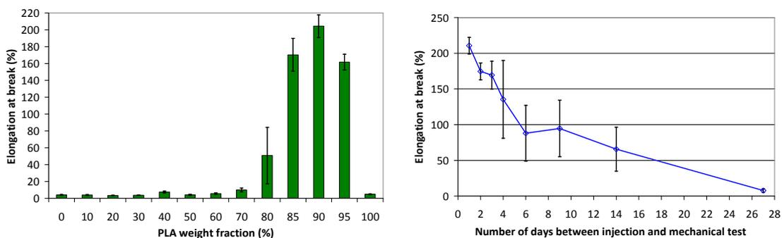
Fig. 2. a) Elongation at break as a function of PLA weight fraction in the PLA/PHBV blends and
