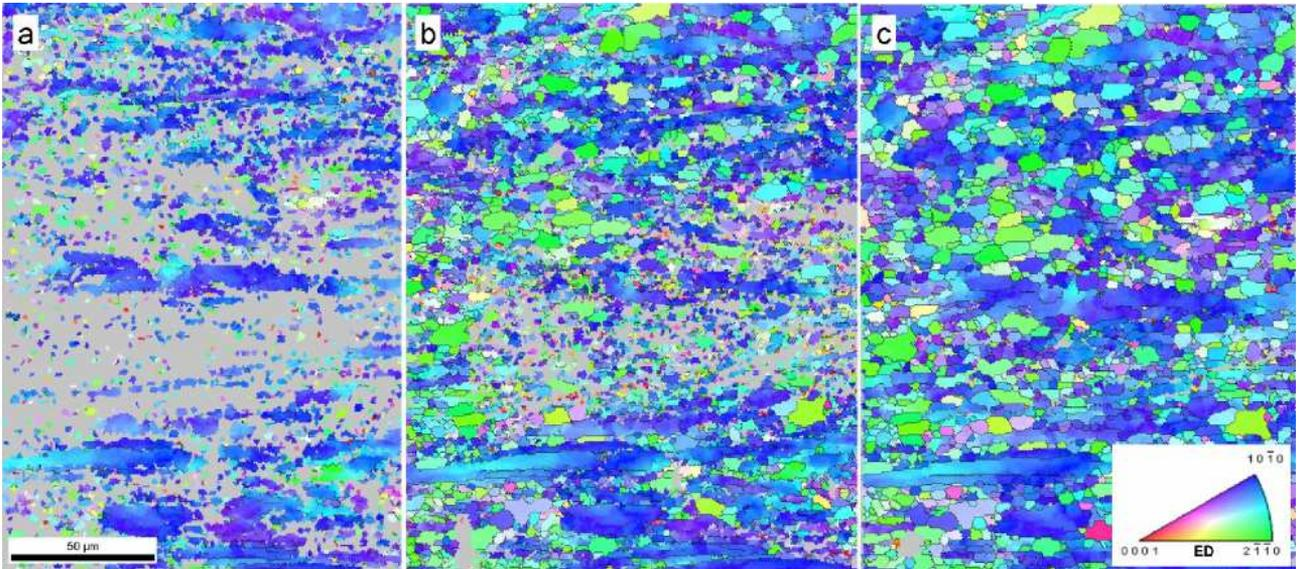
**Figure 3.** Recrystallization sequence of a Zy4 sample. a) initial state (hot-extruded at 685°C and cooled down rapidly). Microstructure after b) two, c) three, successive 5s in-situ annealing treatments at 750°C. Extrusion direction is horizontal, radial direction vertical, the color code defined on the inverse pole figure refers to the extrusion direction. The grey pixels are those for which the orientation could not be reliably determined. EBSD scan step size: 0.75μm.
