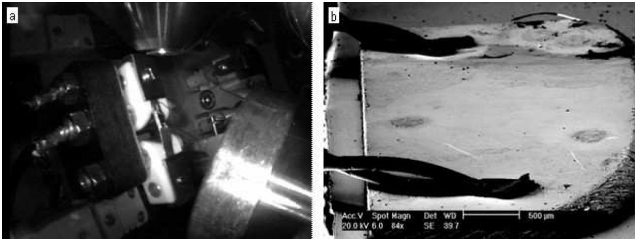
Figure 1. a) Heating stage mounted in the SEM chamber, tilted to 70° to suit EBSD settings. b) Thermocouples welded on the sample which itself is welded on the Ta plate.
