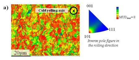
Color code of EBSD scan : angle between < 110> and z axis (rolling axis) from 0°(red) to 50°(blue)
