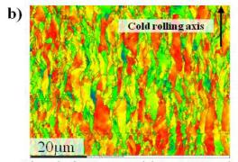
Color code of EBSD scan: angle between < 110> and x ory axis (radial direction of the tube) from 0°(red) to 50°(blue)
