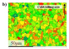
Color code of EBSD scan: angle between < 110> and x ory axis (radial direction of the tube) from 0 °(red) to 50 °(blue)
