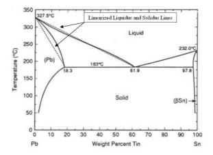
Figure 1. Phase diagram of the Pb-Sn alloy
