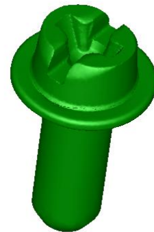
Figure 8: final Philips shape after forging
