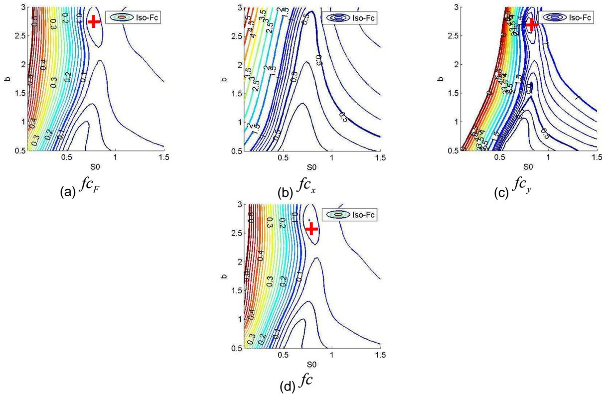
Figure 4 : sensitivity analysis of damage law parameters by kriging response surfaces, evolution of the three objective functions based on: (a) load-displacement, (b) displacement field  $U_x$  in the tensile direction, (c) displacement field  $U_y$  in the transverse direction, (d) total objective function
