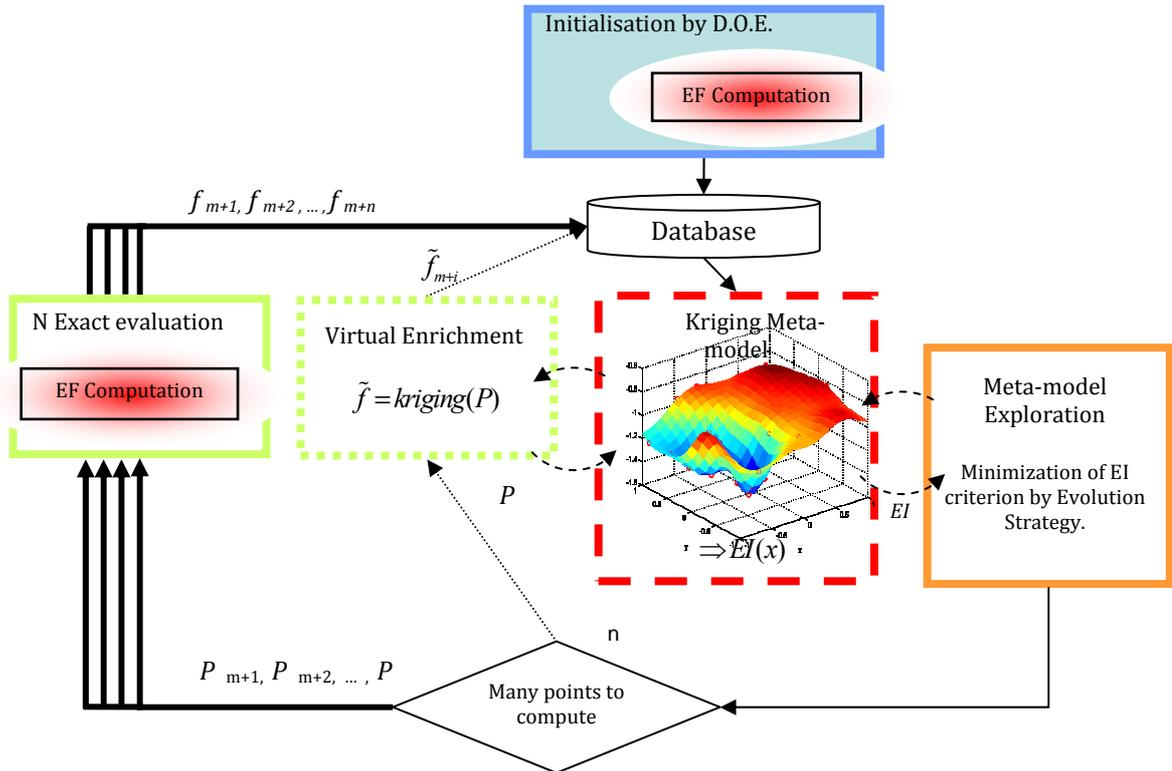
Figure 2: Flowchart of parallel extension of the EGO algorithm implemented in the MOOPI software
