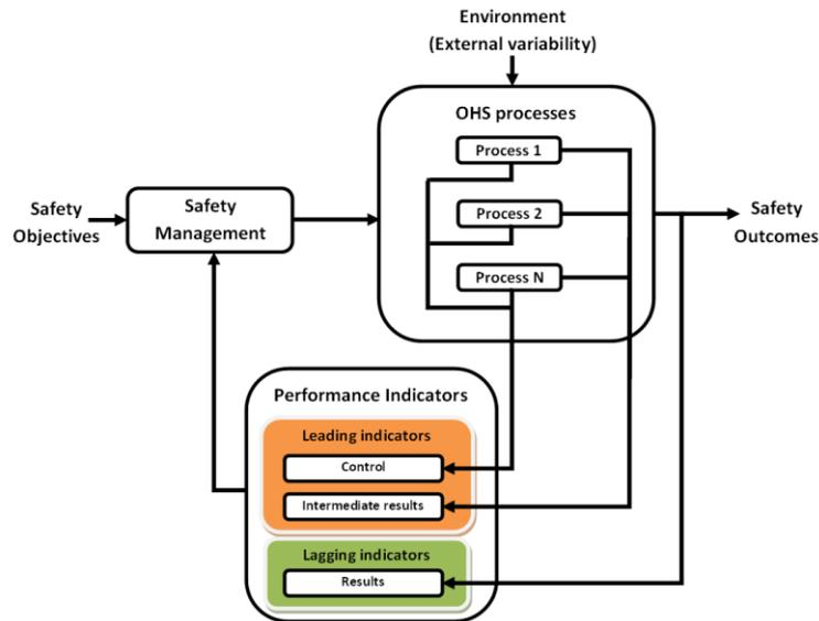
**Figure 3:** Leading and lagging indicators in an OHS management system
