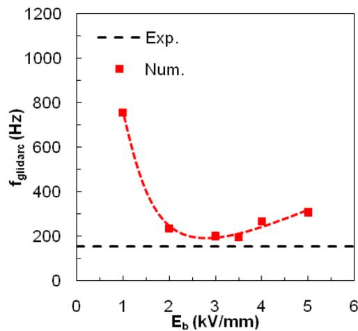
**Figure 4.** Influence of  $E_b$  on glidarc frequency.  $I = 250 \text{ mA}$ .  $Q_{\text{air}} = 0.32 \text{ g.s}^{-1}$ .
