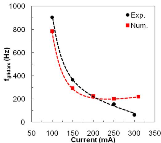
**Figure 13.** Influence of the electrical current on the glidarc frequency.  $Q_{air} = 0.32$  gs<sup>-1</sup>.
