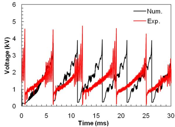
**Figure 7.** Experimental and numerical voltage vs. time.  $I = 0.25$  A.  $Q_{\text{air}} = 0.32$  gs<sup>-1</sup>.
