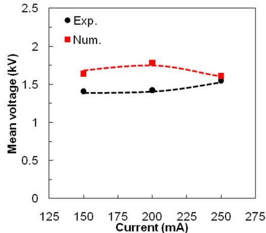
**Figure 14.** Influence of the current on the mean voltage drop.  $Q_{\text{air}} = 0.32 \text{ gs}^{-1}$ .
