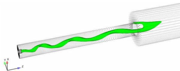
**Figure 9.** Iso-temperature (3000 K) just before breakdown.  $t = 16$  ms.  $I = 0.25$  A.  $Q_{\text{air}} = 0.32$  gs<sup>-1</sup>.
