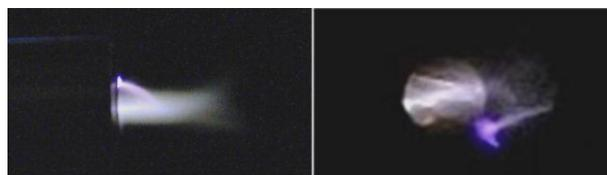
**Figure 8.** Fast camera photograph of the plasma arc at the tip of the nozzle. Left: side view. Right: Front view.  $I = 0.25$  A.  $Q_{\text{air}} = 0.32$  gs<sup>-1</sup>.
