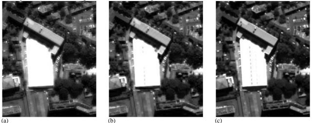
Fig. 9: Excerpt of Pleiades images over Toulouse, France. Red band synthesized with a) ATWT-M3, b) ATWT-M3-MTFadapted, c) reference image. Copyright CNES 2000.
