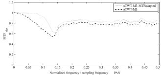
Fig. 7: Modulation transfer function of the images ATWT-M3 and ATWT-M3-MTFadapted relative to the MTF of Pleiades
