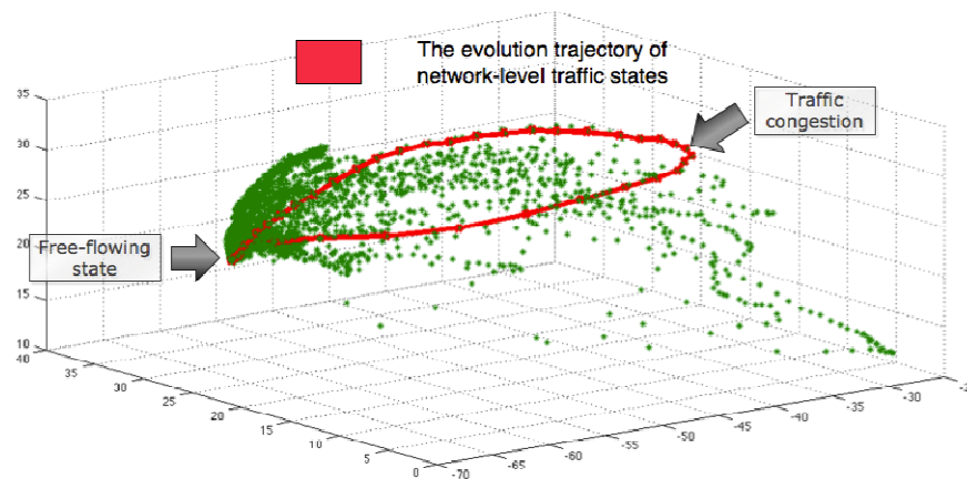
Figure 5. The evolution trajectory of network-level traffic states, projected in 3D-PCA space
