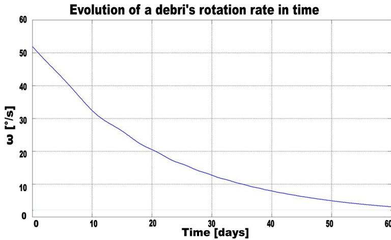
Figure 3: Attitude simulation for the flight 35 H10 stage.
