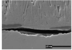
Fig. 3: Interfacial failure in TBCs due to LASAT
