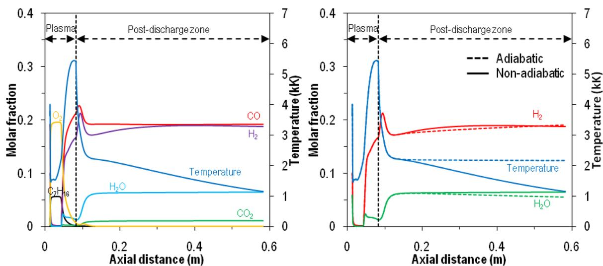
Figure 10. Evolution of the temperature and main species along the nonadiabatic reactor axis for the  $\text{PO}_x$  condition (left) and comparison with the adiabatic model (right).  $P = 1000 \text{ W}$ .
