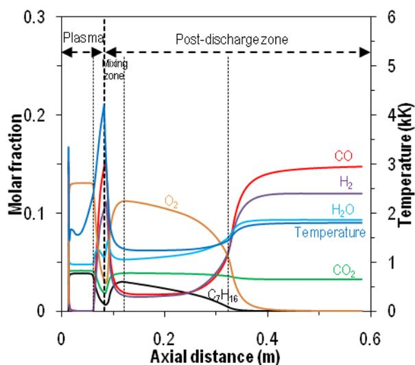
Figure 9. Evolution of the temperature and main species along the reactor axis for the  $\text{NO}_x$  trap application.  $P_{\text{plasma}} = 1000 \text{ W}$ .
