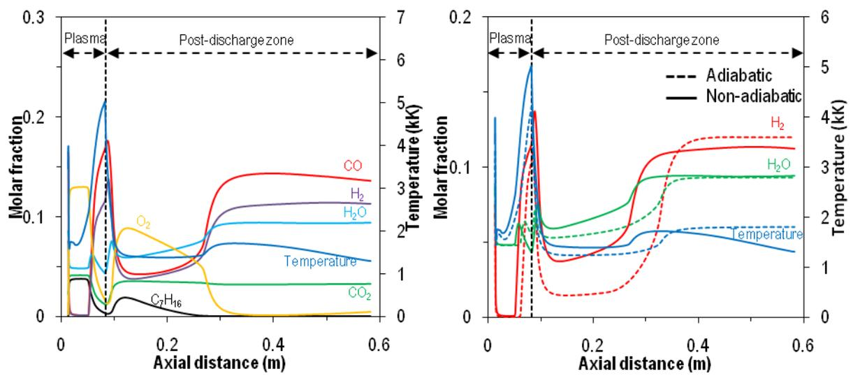
Figure 11. Evolution of the temperature and main species along the nonadiabatic reactor axis for the  $\text{NO}_x$  trap regeneration condition (left,  $P = 1200 \text{ W}$ ) and comparison with the adiabatic model (right).
