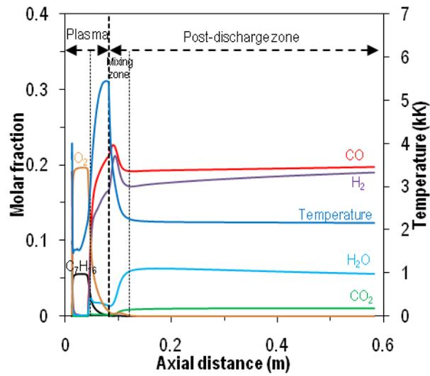
Figure 4. Evolution of the temperature and main species along the reactor axis.  $P_{\text{plasma}} = 1000$  W.
