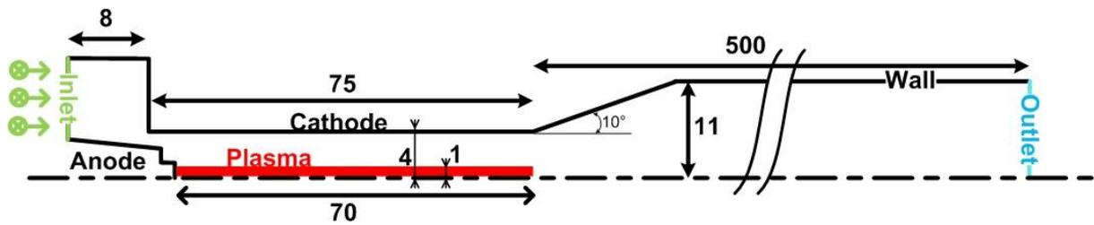
Figure 1: Scheme of the computational grid (unit: mm).
