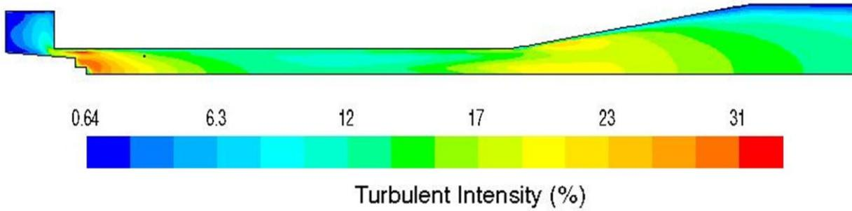
Figure 7. Turbulent intensity in the plasma zone and mixing zone. PO<sub>x</sub> condition.
