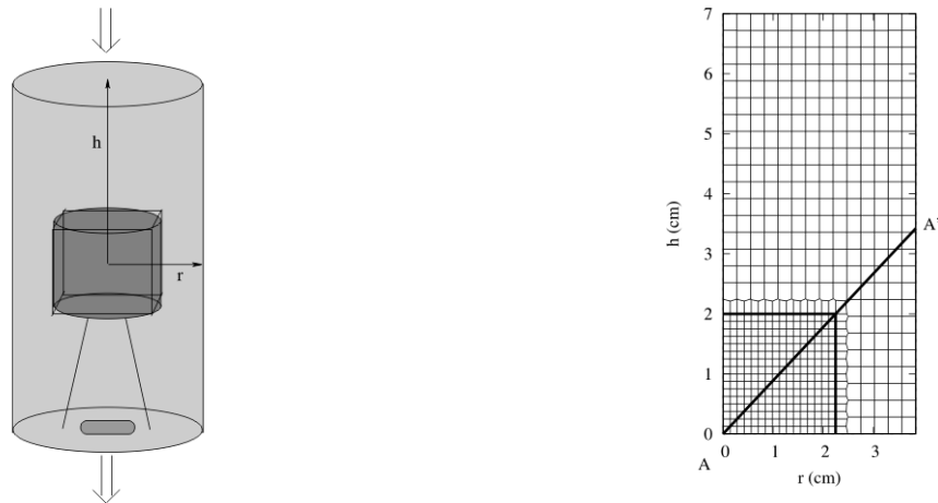
Fig.1. Zoom on the reactor zone of the dynamic leaching test applied to the monolithic waste (left) and one of the calculation grids assuming cylindrical symmetry (right).
