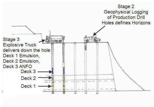
Figure 65. Geophysical Logging & Blast holes Charging Section.
