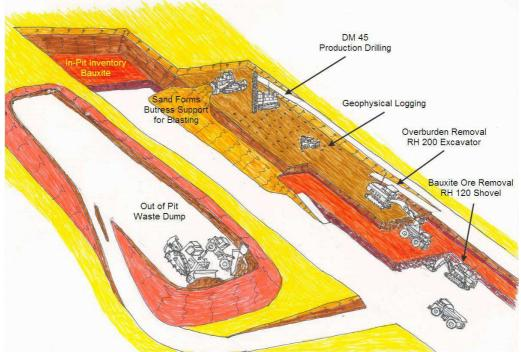
Figure 68. Overall View of Mining Activates.
