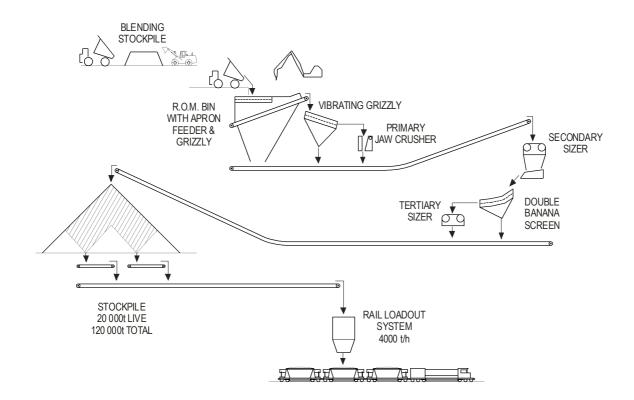
Figure 69. Mine Processing Facility Flow Sheet.
