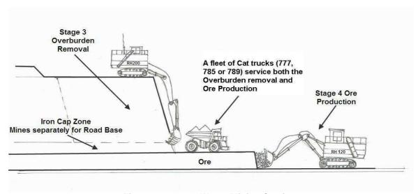
Figure 67. Ore & Waste Mining Section.
