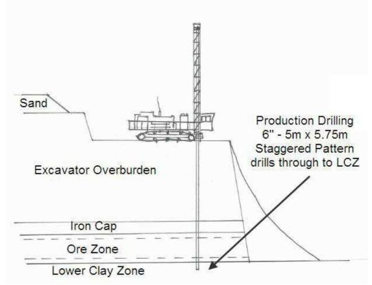
Figure 64. Production Drilling Section.
