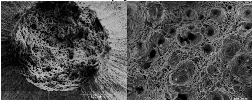
Figure 13: Fracture surface of the crept sample after 2837h (229.6 MPa, 550°C).
