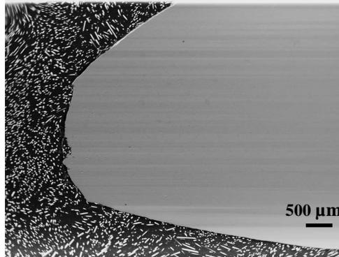
*Figure 14: Necking area of a crept sample (240 MPa, 550°C).*
