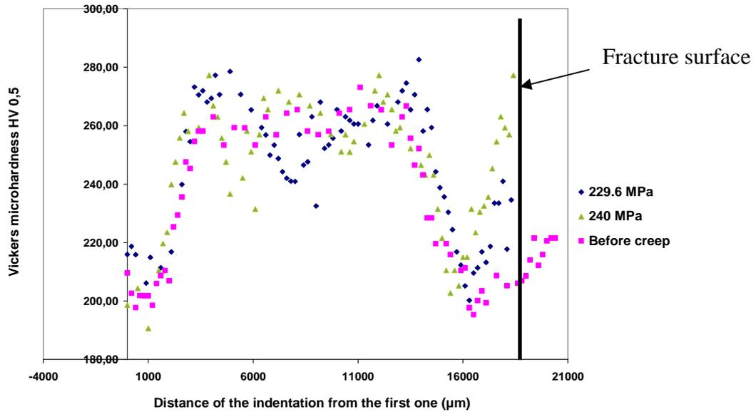
Figure 17: Cross-weld microhardness profiles of two crept specimens
