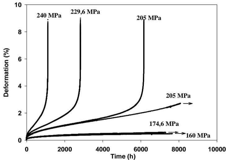
Figure 9: Creep curves at 550°C.
