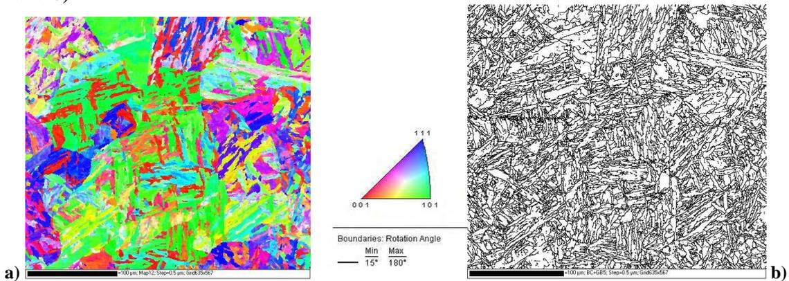
**Figure 5: EBSD orientation map a) and boundary map (misorientation  $>5^\circ$ ) b) of the base metal.**
