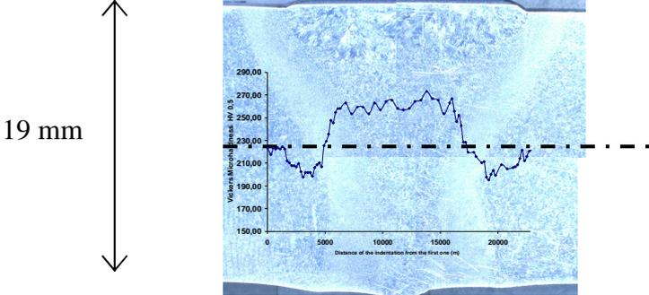
Figure3: Cross-weld microhardness profile combined with observations of the welded joint.
