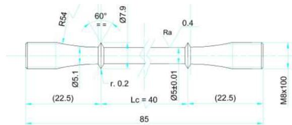
Figure 1: Scheme of creep specimen geometry.
