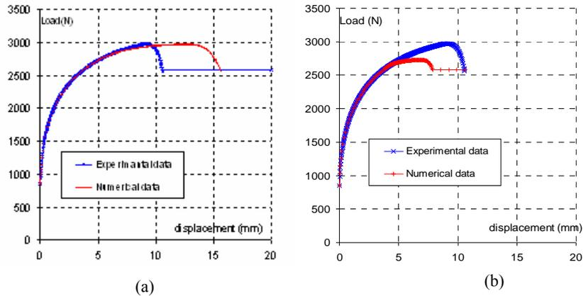
**FIGURE 2.** Tensile test load-displacement curves, (a) numerical fracture appears for a larger displacement value than for the experimental curve, (b) numerical fracture appears for a smaller displacement than the experimental fracture displacement
