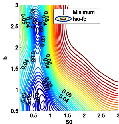
**FIGURE 3.** Evolution of the cost function computed with the load-displacement curve for two damage parameters  $b$  and  $S_0$  - illustration of the non-uniqueness of the inverse problem (Aluminum EN AW-5774[AlMg3])
